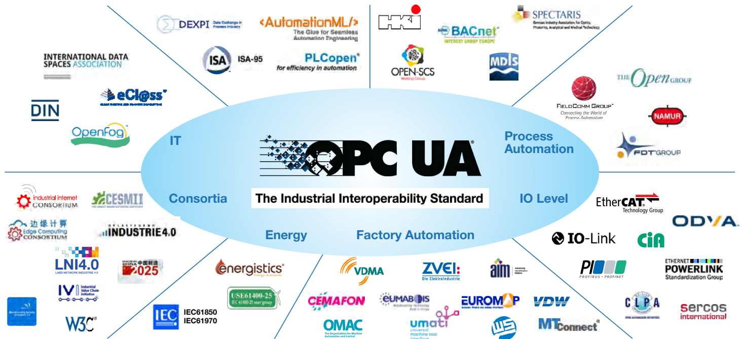
Graphic: The OPC Foundation closely cooperates with organizations and associations from various branches. Specific information models of other standardization organizations are mapped onto OPC UA and thus become portable. The organizations define „what“ shall be communicated. OPC UA delivers how through its secure and effective transport and offers access privileges and generic interoperability.
