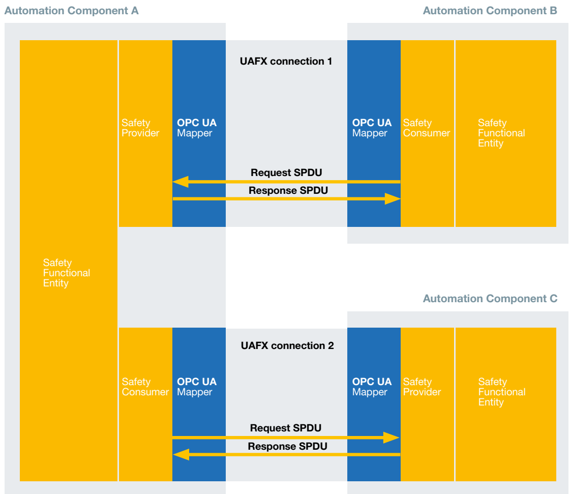
Figure 19: Safety connections between Automation Components
